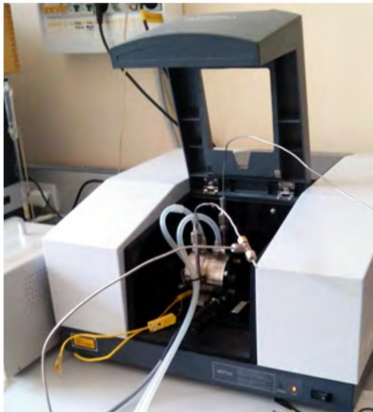
High-temperature flow IR cell with gas pathway 5 mm in sample chamber of spectrometer IR-Prestige (Shimadzu) for a temperature range of 25 - 400 °C
