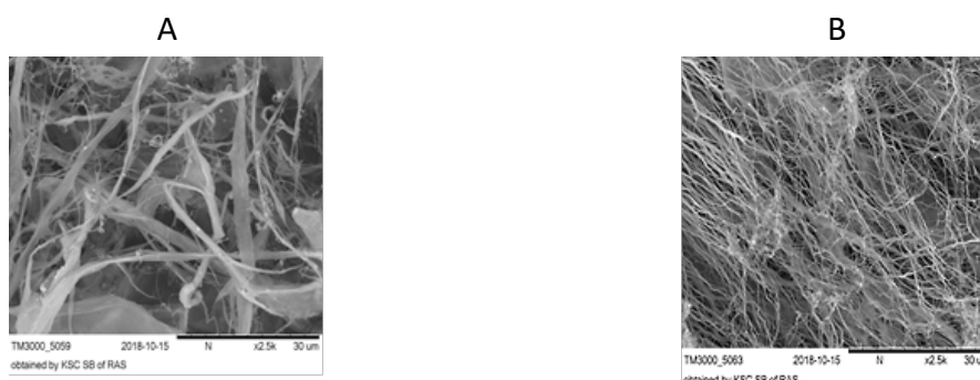
Fig. 2. SEM-images of the samples MFC (A) and NCC (B) obtained from larch wood. (magnification 2000 times)
