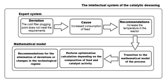
Figure 1 - Algorithm of application of the intellectual system of the catalytic dewaxing process
