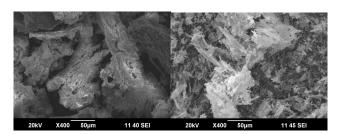
Fig. 1. SEM images of CZ(CTAB) (left) and CZ(SD)
