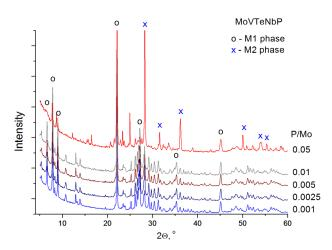
Fig.1. XRD patterns of the MoVTeNbP catalysts
