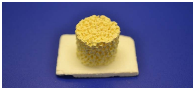
Figure 1. Alumina foam with catalytically active platinum layer at the surface
