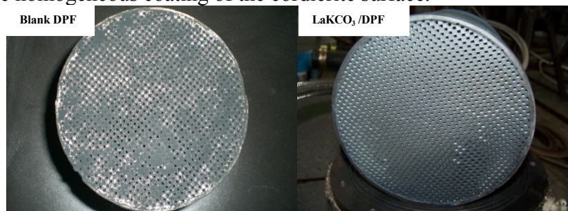
Fig.1. Photographs of the blank DPF compared with the one coated with perovskite LaKCoO 3 catalyst after the bench testing.
