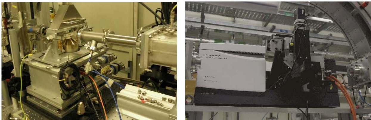
Fig. 1. a) Capillary reactor with hot air blower, on the B18 beamline b) FTIR spectrometer with Da Vinci arm and Harrick DRIFTS cell attached, on the B18 beamline.
