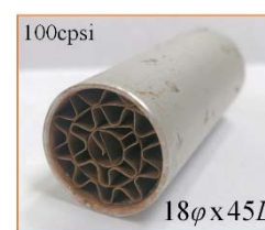
Fig.1 Overview of the prepared honeycomb-type Ni-based catalyst.
