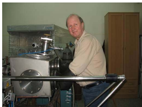
Figure 1. Download the sample into the SPECS spectrometer using «home made» glove box.
